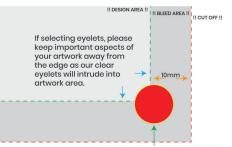
This is the clear rivet hole, it is 12mm in diamater. It must be positioned away from the edge toward the design area, to ensure the corflute signs longevity.
